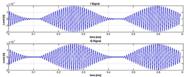
Fig. 11 – Measurement of an AM-Modulation Signal as I-Q Visualization.
