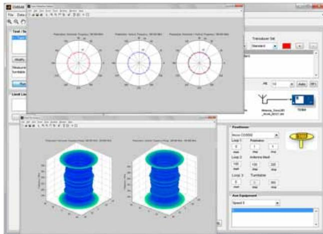
Fig. 13 – Screenshot EMI 64k Software Suite - Radiation pattern in 2D and 3D.
